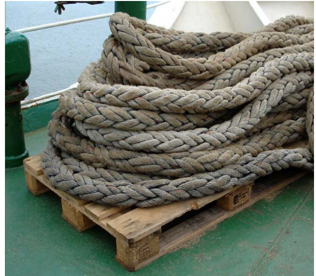
Ropes correctly stowed off deck
