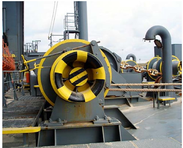
Mooring station with effective hazard markings
