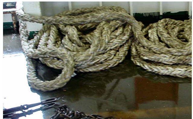
Ropes badly stored on wet deck
