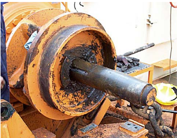
This windlass drum suffered bearing damage and is being overhauled
