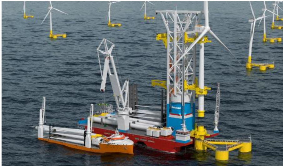
Figure 19 – Floating WIV installing on a floating site with motion compensation
