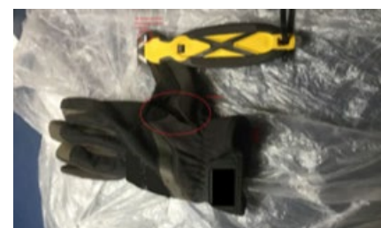
Incident 1: Damaged alternative cutting device and cut glove
