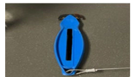
Incident 2: Exposed blade on alternative cutting device
