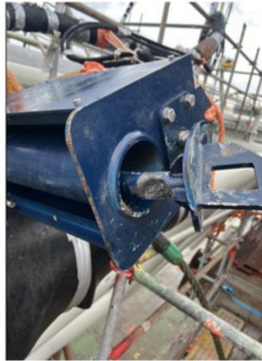
Bent connection plate
