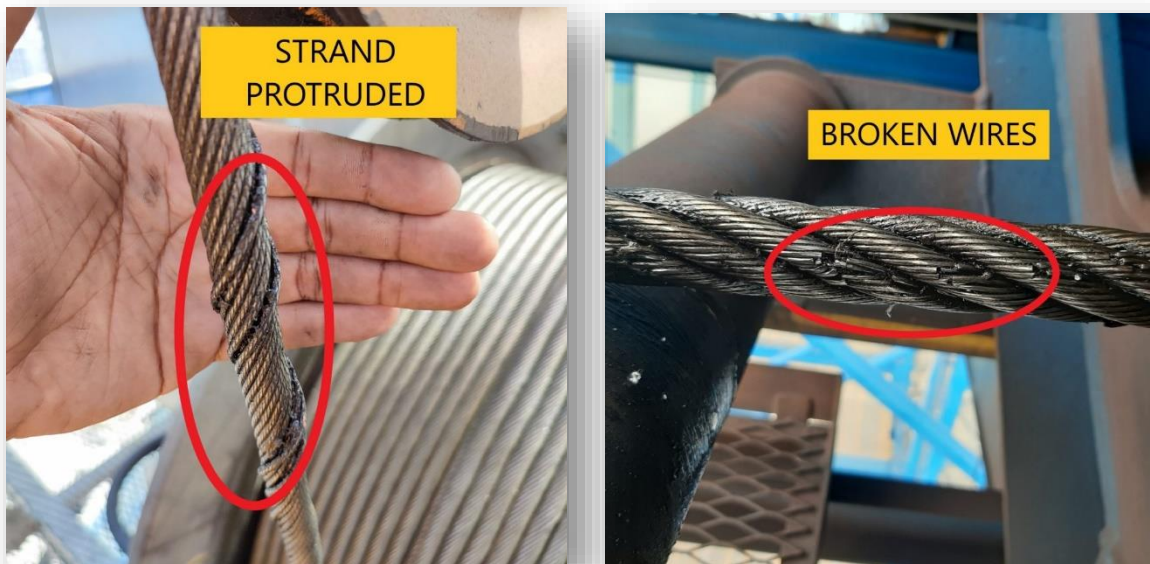
Figures 7 – Example Wire Rope Failure Modes
