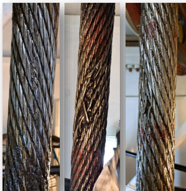
Figure 16 – Damage to the auxiliary hoist rope
