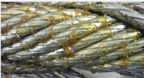
Figure 30 – Bio-grease / wrong lubrication & excess lubrication
